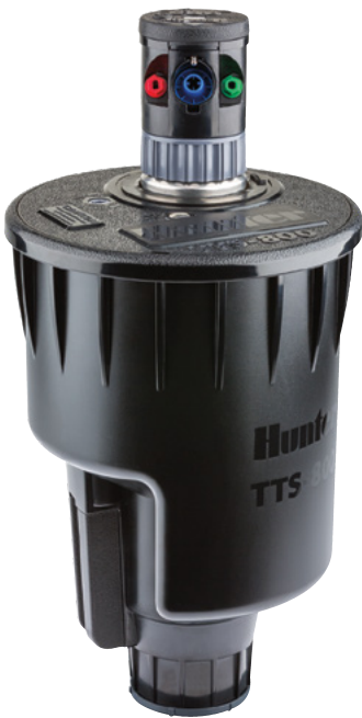
TTS-885 Pop-up height: 9.5 cm Overall height: 30 cm Flange diameter: 18 cm Female inlet: 1½" (40 mm) Acme
