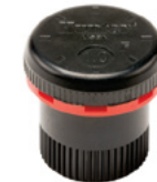
MSBN-10H/10F Flow: 0.23 m 3 /hr; 3.8 l/min
