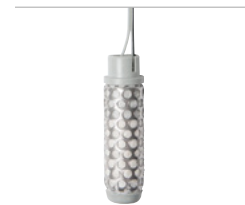
SC-PROBE Soil Moisture Sensor Probe Diameter: 2.5 cm Height: 8.3 cm Controller to probe: 30 m maximum 1 mm 2 direct-burial wire
