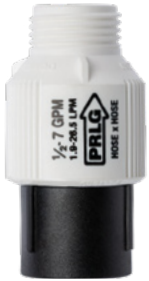
PRLG - Pressure Regulator Landscape Grade Width: 41 mm Length: 79 mm ¾" FHT inlet x ¾" MHT outlet
